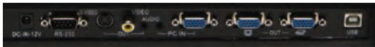
Rear ports enable connections to a variety of equipment - from computer monitors to projectors
